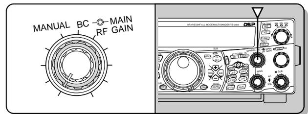
Depending on the type and gain of your antenna, and the condition of the band, you may also prefer leaving the **MAIN RF** control turned counterclockwise by the same amount rather than turning it fully clockwise. When using FM mode, always set the **MAIN RF** control fully clockwise.
