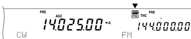
Or, if you would like to transmit and receive on the MAIN band while adjusting the sub receiver functions, simply press **[CTRL]**. Only the CTRL icon moves from the main transceiver display to the sub display. The "PTT" icon remains on the main transceiver display. With this setup, you can continue receiving and transmitting on the main transceiver VFO frequency(ies) while you are making adjustments to the sub-receiver functions.
