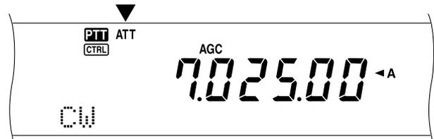
The ON/OFF setting will be automatically stored in the current band. Each time you select the same frequency band, the attenuator setting will be automatically recalled.
