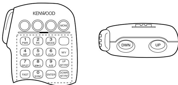
Each time you press a key, the Commander will automatically enter transmit mode and send the corresponding control command to the Transporter.
