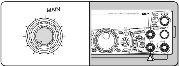
**Note:** The position of the **MAIN AF** control does not affect the volume of beeps caused by pressing keys nor the CW transmit sidetone. The audio level for Packet operation is also independent of the **MAIN AF** control setting.
