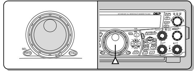
You may prefer directly entering a frequency using the numeric keypad if the desired frequency is far from the current frequency. Press **[ENT]**, then press the numeric keys as necessary. For details, see "Direct Frequency Entry" {page 37}.
