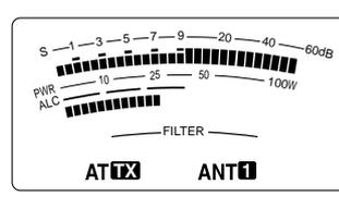
**AM:** While speaking into the microphone, adjust the **MULTI/ CH** control so that the calibrated power meter slightly reflects to your voice level.
