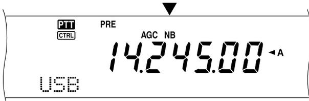
You can further adjust the Noise blanker level from 1 to 10. The default level is 6.
