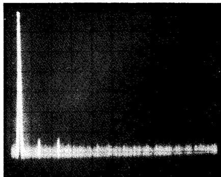
Fig 2—Worst-case spectral display of the ICOM IC-781. Horizontal divisions are each 2 MHz; vertical divisions are each 10 dB. Output power is approximately 156 W at 1.9 MHz. All harmonics and spurious emissions are at least 63 dB below peak fundamental output. The IC-781 complies with current FCC specifications for spectral purity.
