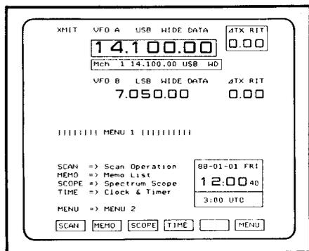
Fig 1—This view of the Menu 1 screen on the IC-781's multifunction CRT gives a hint of the variety of information it can display on its 17 different menus.
