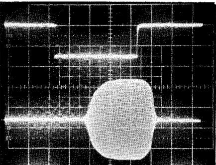
Fig 4—CW-keying waveforms for the ICOM IC-781 in the full-break-in mode. The lower trace is the RF envelope; the upper trace is the actual key closure. Each horizontal division is 5 ms. The IC-781's CW keying is extremely good.
