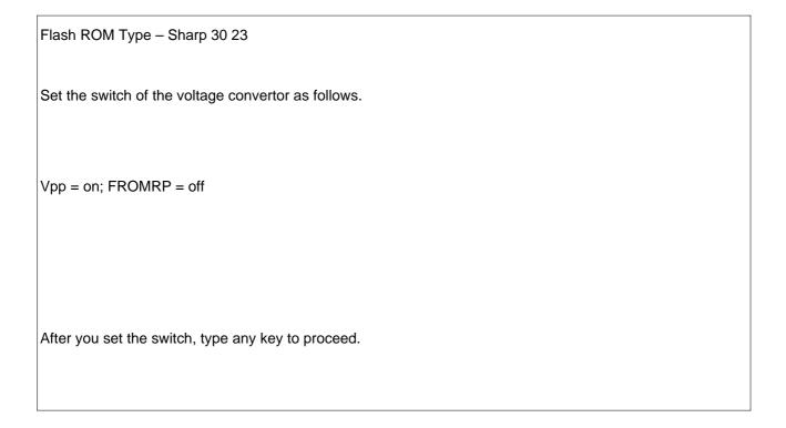
The user is requested to set the switches on the Level Shifter to the settings displayed.
