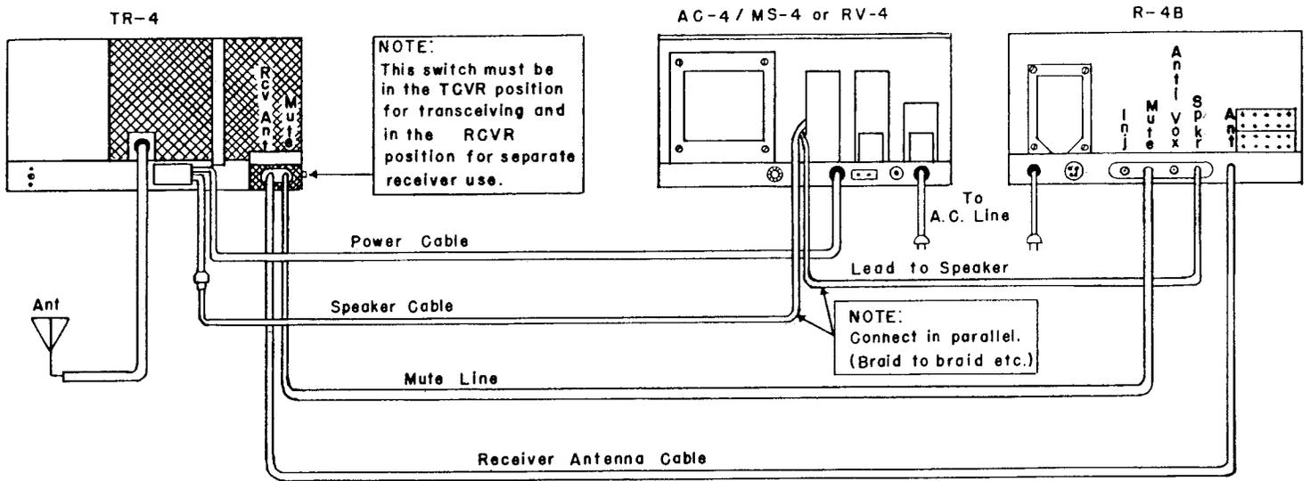
FIG. 1 USING THE R-4B WITH THE TR-4 TRANSCEIVER
