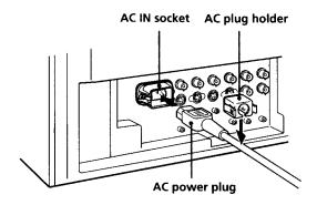
**2** Slide the AC plug holder over the cord until it connects to the attached holder.
