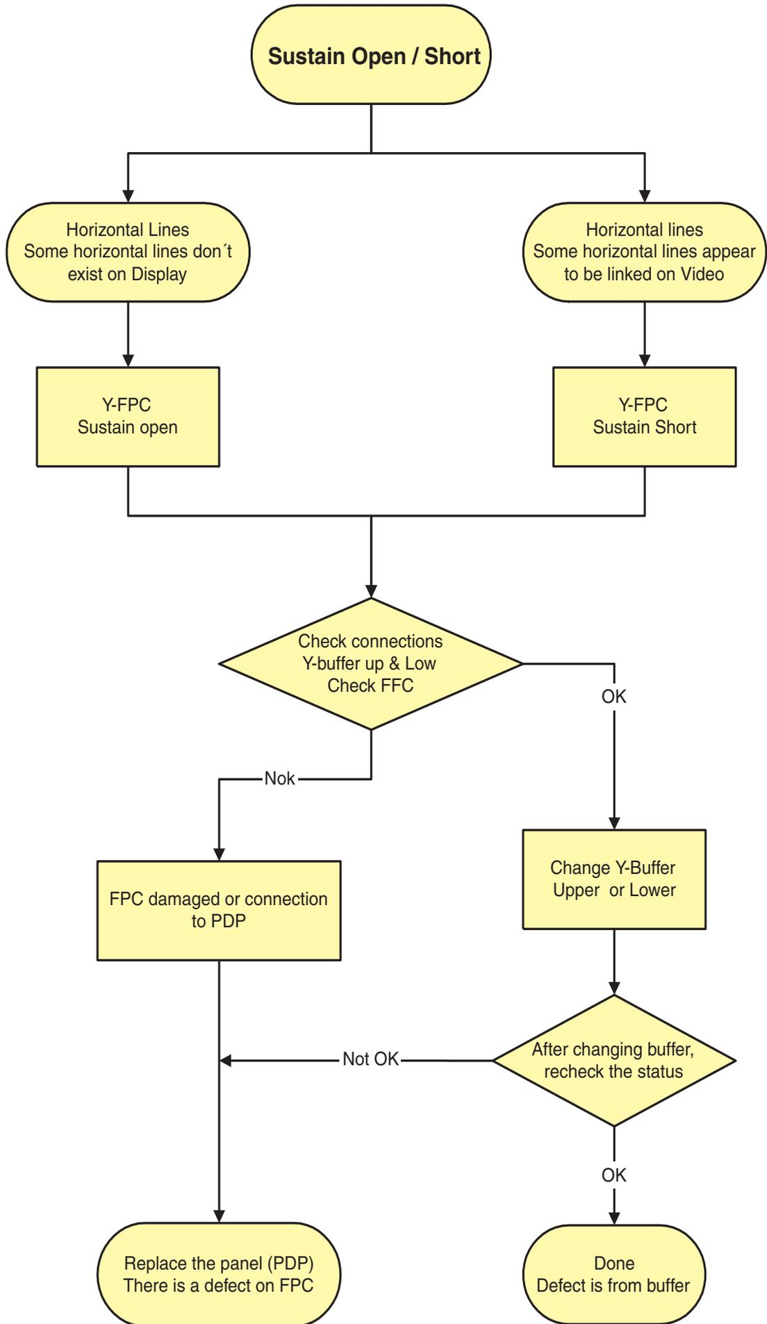
Figure 5-15 Fault symptom: "Sustain open / short"
