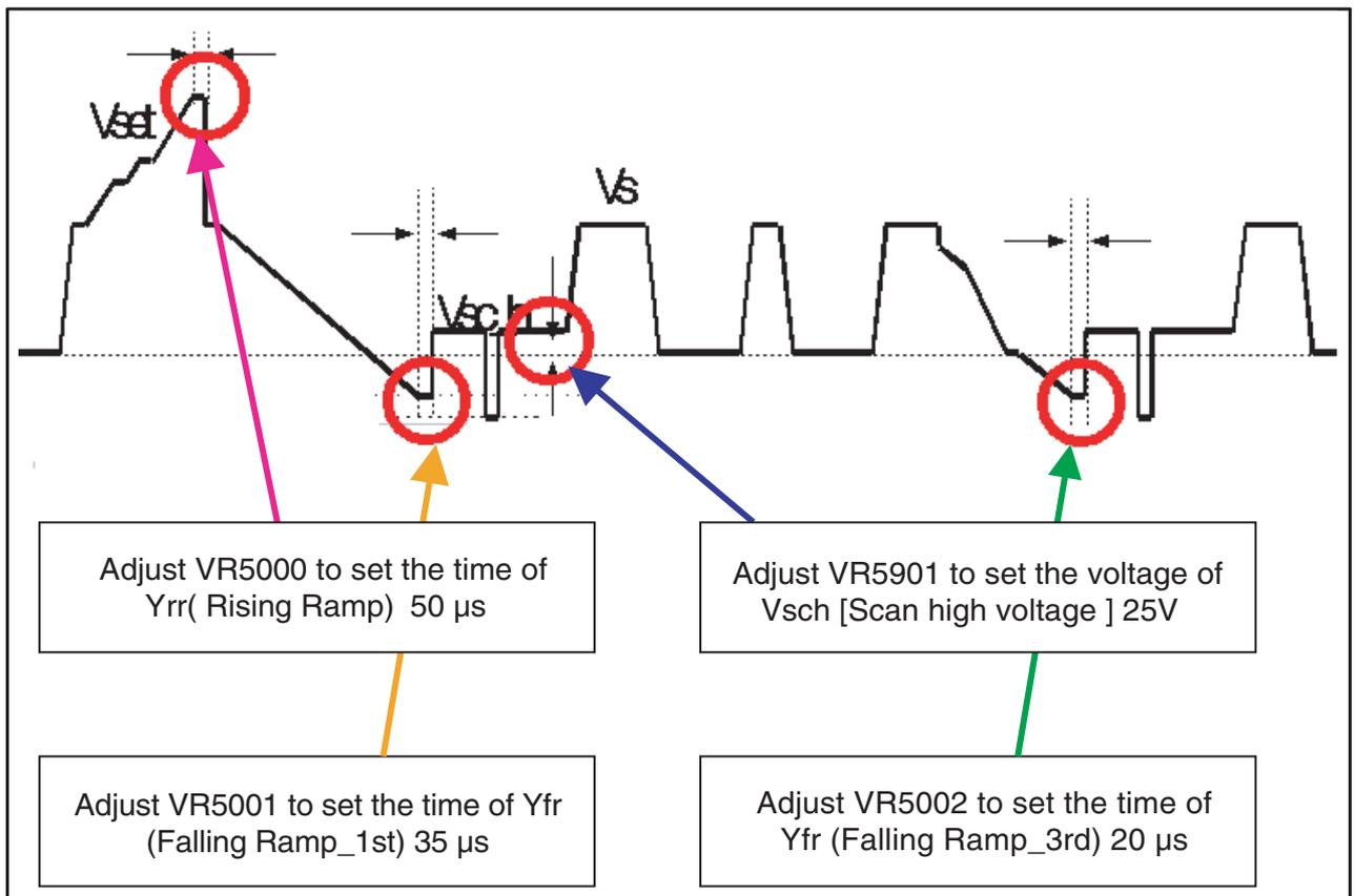
Figure 8-37 TCP ramp waveform inclination adjustment (Y-Board)
