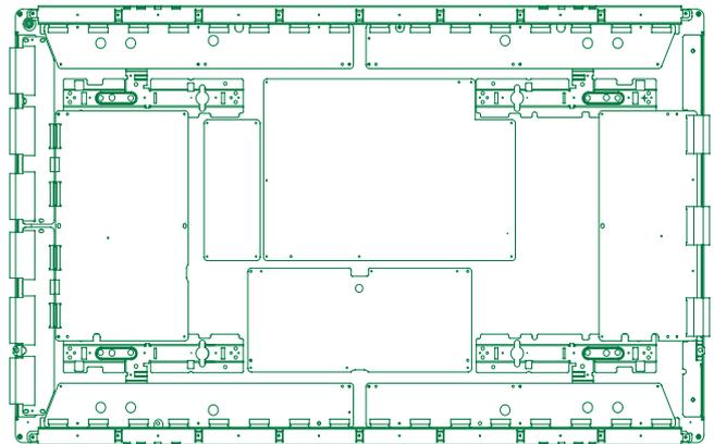
Figure 1-10 Points of screw mount (42" HD v3)
