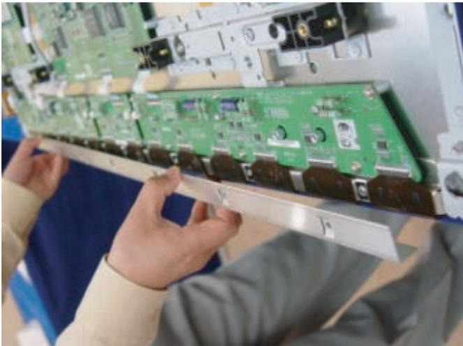
Figure 4-9 Photo 1 - Heatsink removal
