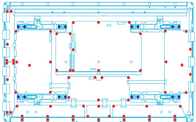
Figure 1-6 Points of screw mount (42" SD v3)
