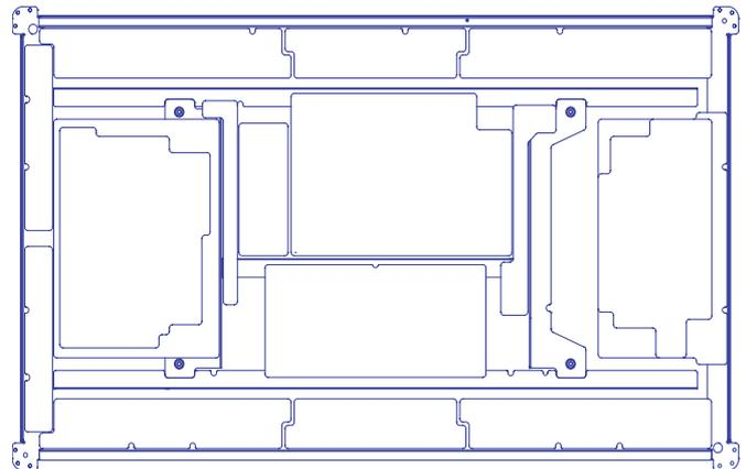
Figure 1-14 Points of screw mount (50" HD v3)
