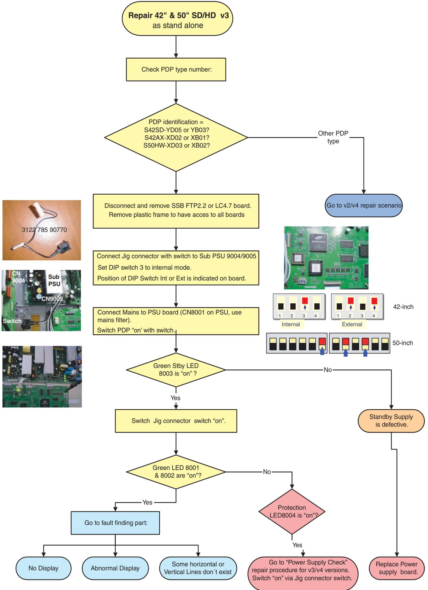
Figure 5-7 Repair scenario 42"/50" SD/HD v3 stand alone panels
