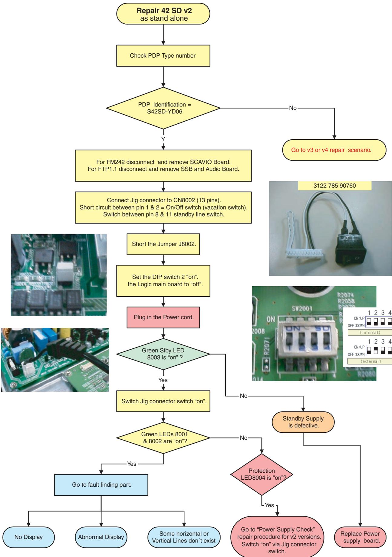
Figure 5-6 Repair scenario v2 stand alone panels
