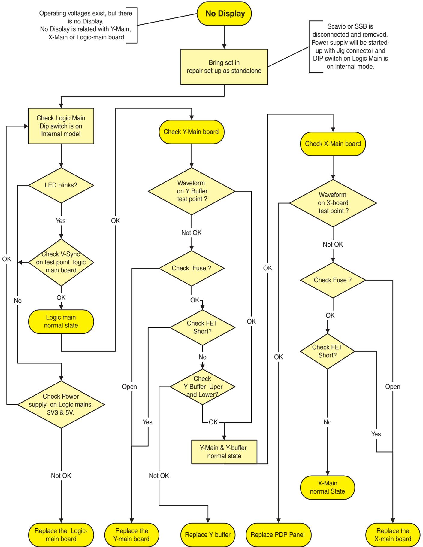
Figure 5-13 Fault symptom: "No Display"
