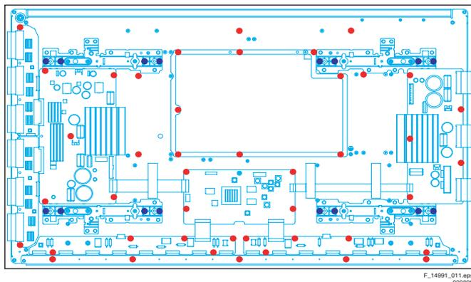
Figure 1-12 Points of screw mount (42" HD v4)
