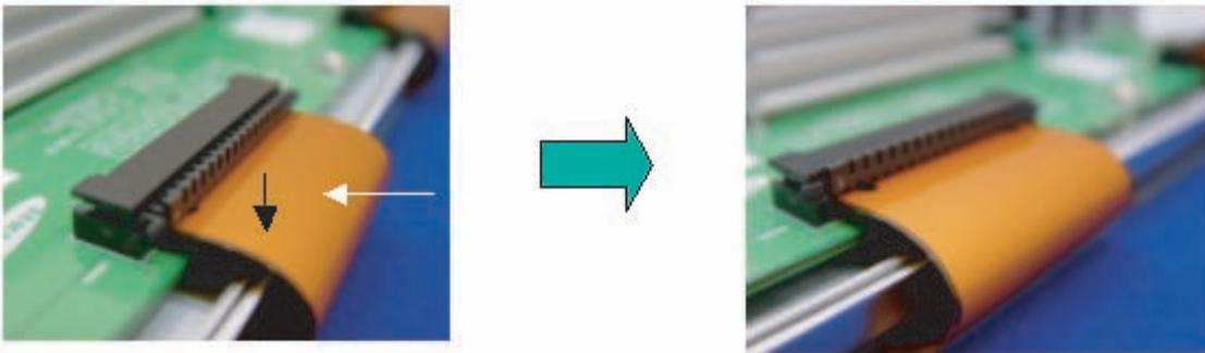
Figure 4-4 Re-assembly FCC of X-main board
