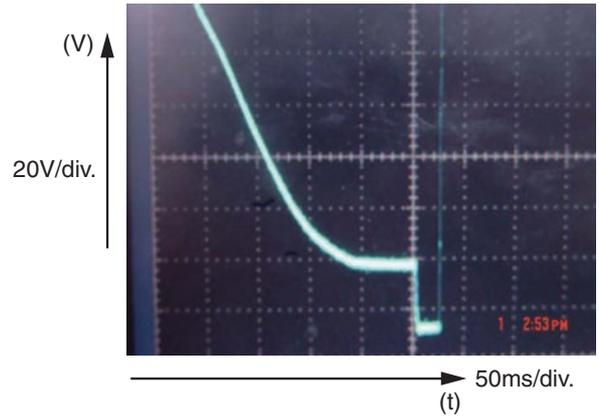
Figure 8-17 Falling ramp
