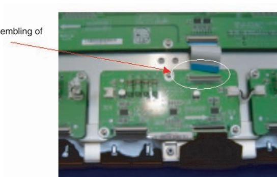
Figure 4-8 Dis- and re-assembly of FFC
