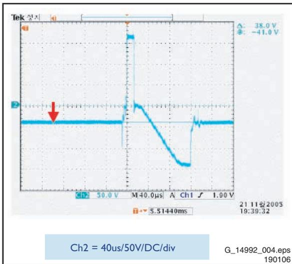
Figure 8-4 Y-scan H waveform (Y-Board)
