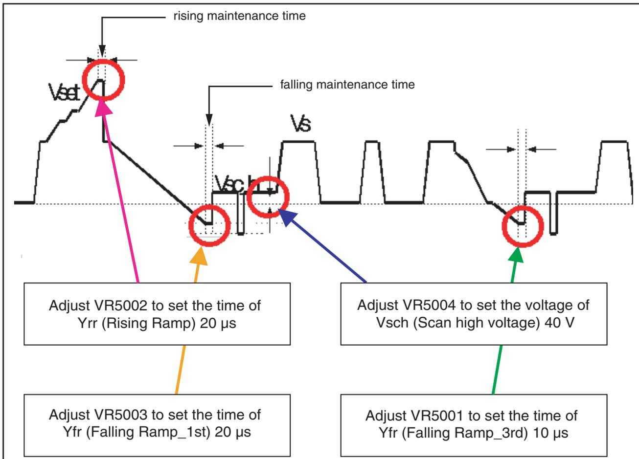
Figure 8-23 TCP ramp waveform inclination adjustment (Y-Board)
