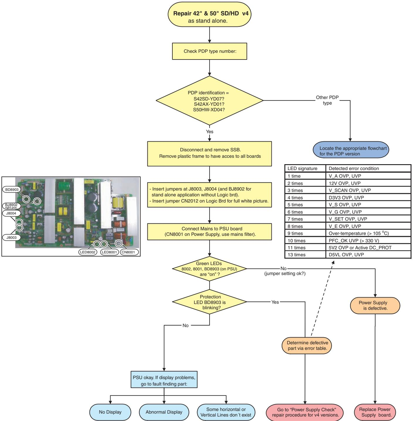
Figure 5-9 Repair scenario 42"/50" SD/HD v4 stand alone panels
