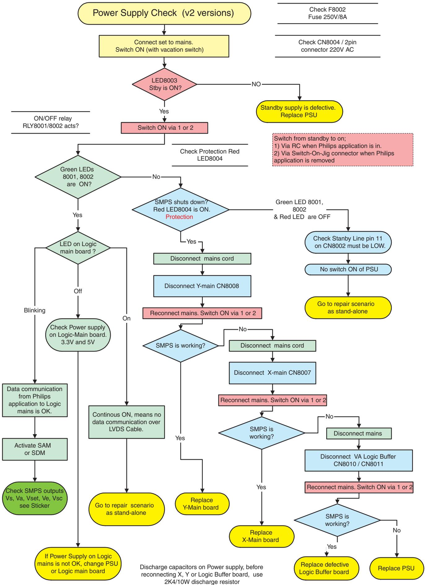
Figure 5-10 Power Supply Check for v2 models
