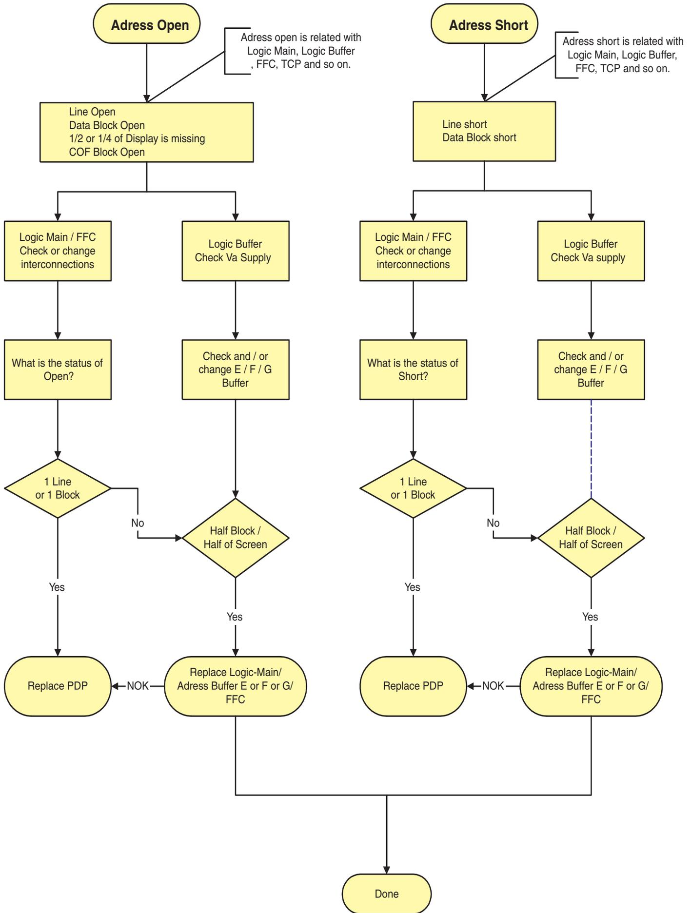
Figure 5-16 Fault symptom: "Address open / short"
