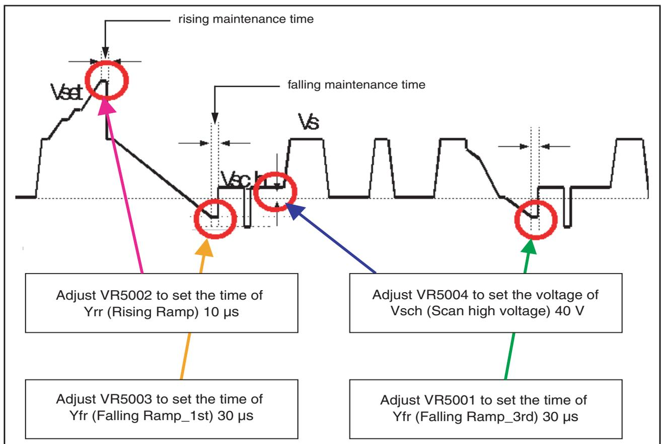
Figure 8-15 TCP ramp waveform inclination adjustment (Y-Board)
