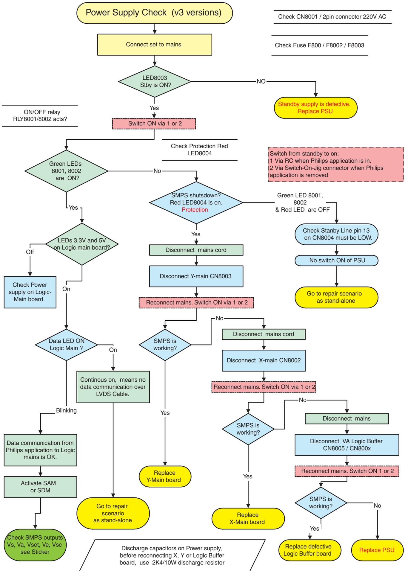
Figure 5-11 Power Supply Check for v3 models
