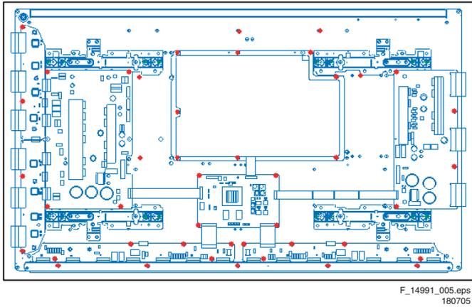
Figure 1-8 Points of screw mount (42" SD v4)
