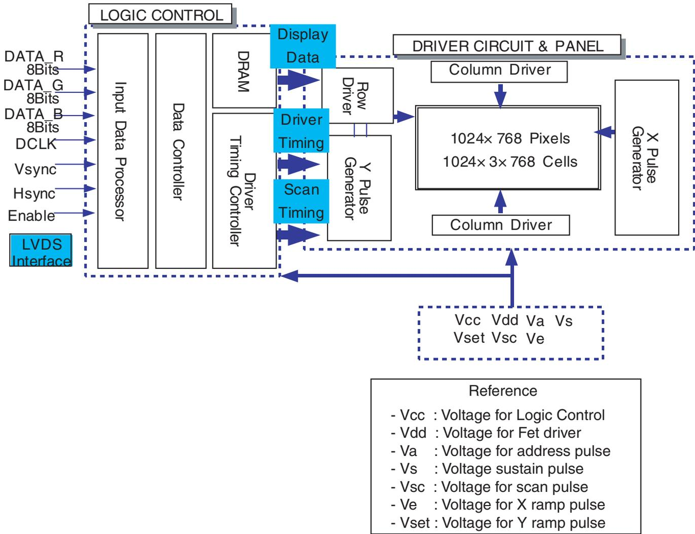
Figure 6-5 Block diagram (42" HD v3)
