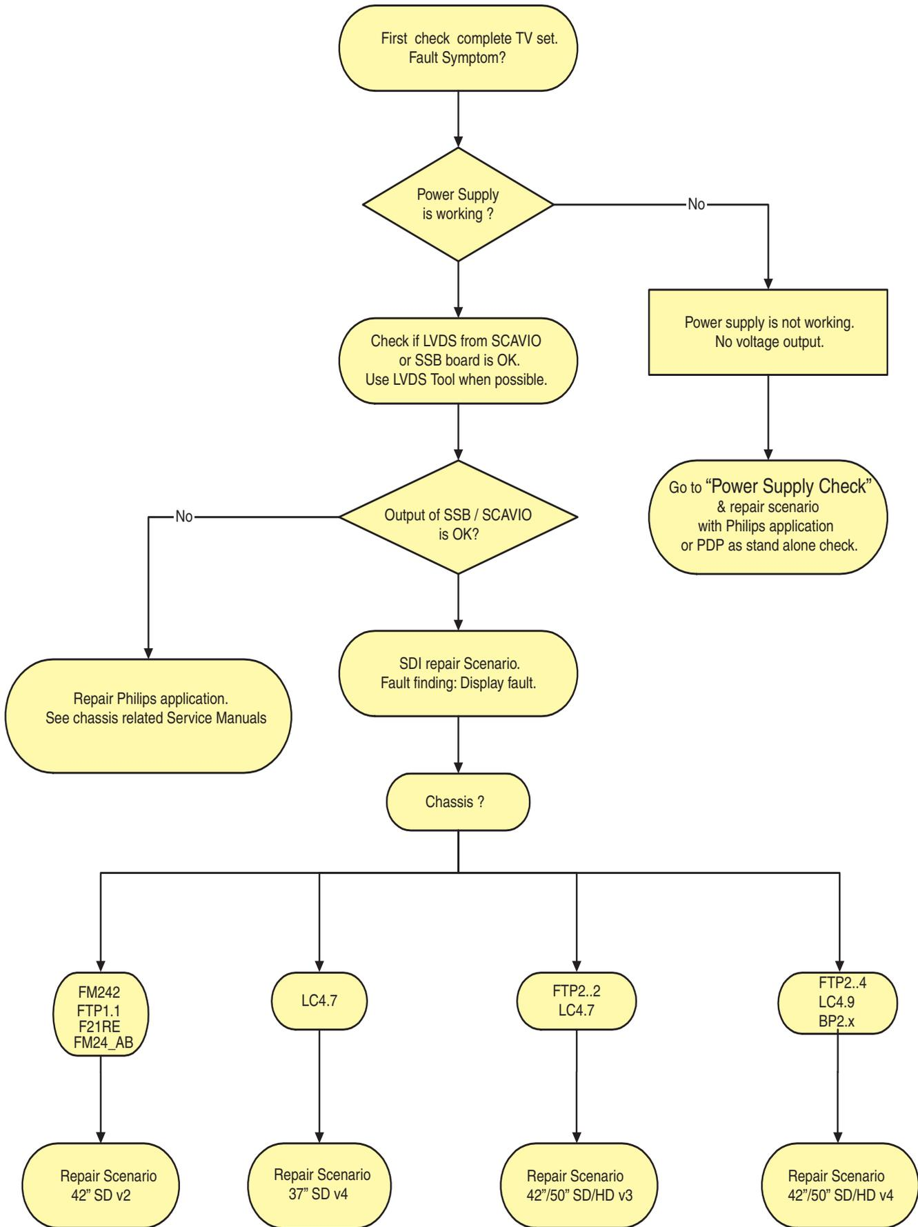
Figure 5-4 Which repair scenario?
