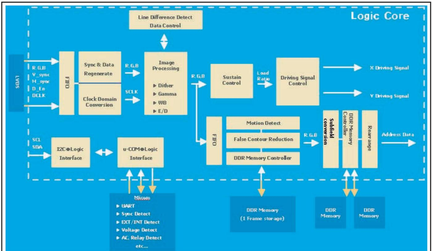
Figure 6-8 Block diagram (50" HD v4)
