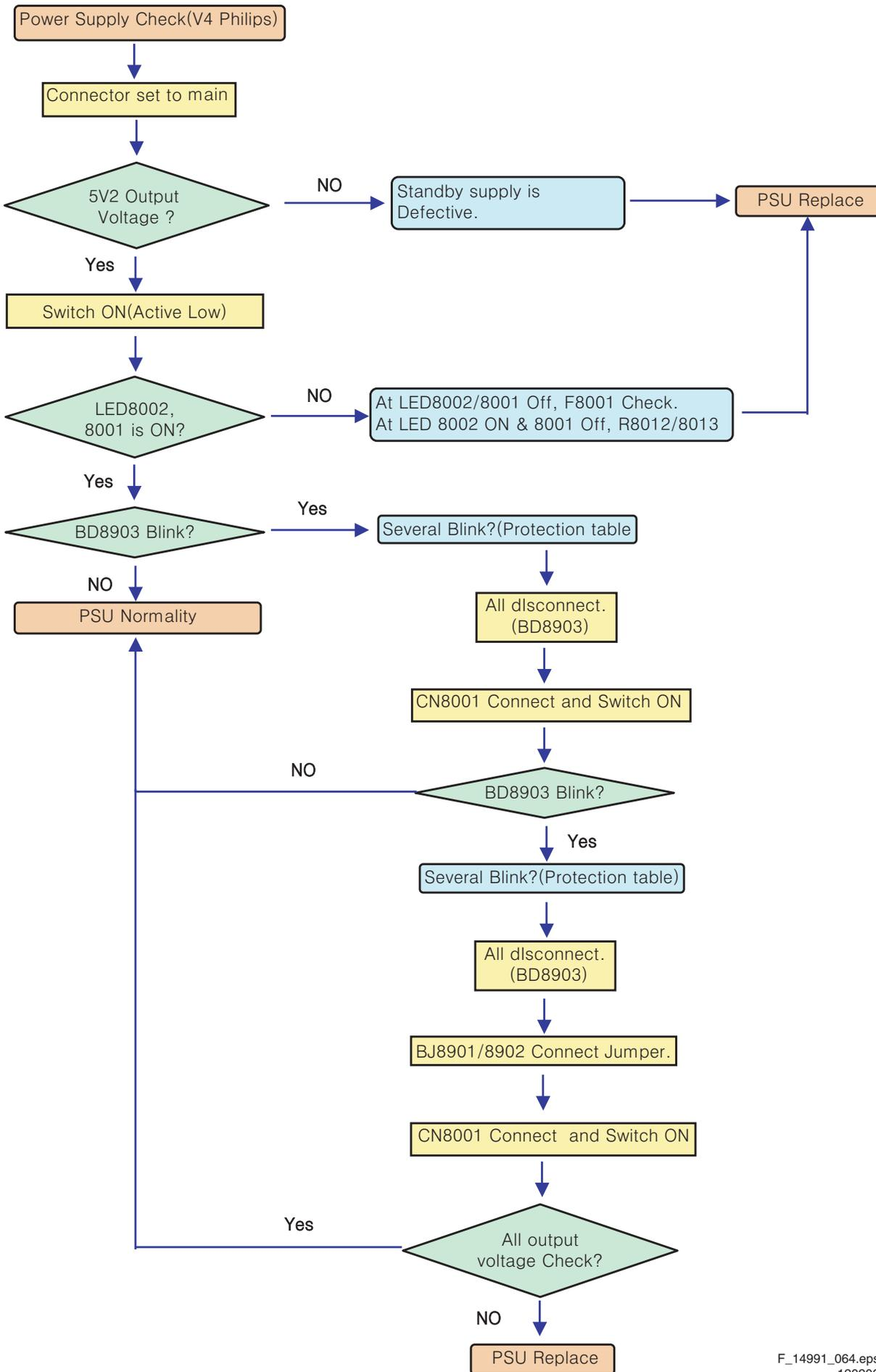
Figure 5-12 Power Supply Check for v4 models
