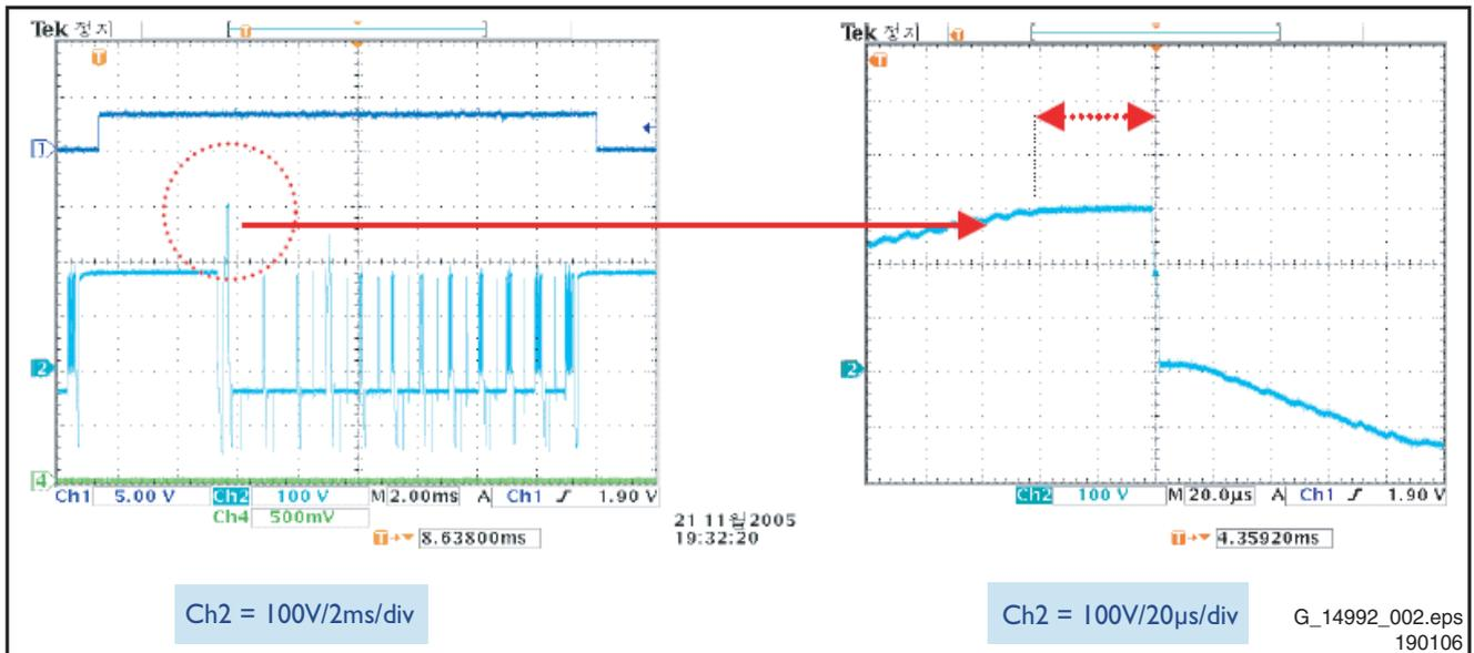
Figure 8-2 Rising ramp flat time adjustment (Y-Board)
