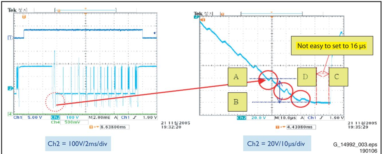
Figure 8-3 Falling ramp flat time adjustment (Y-Board)
