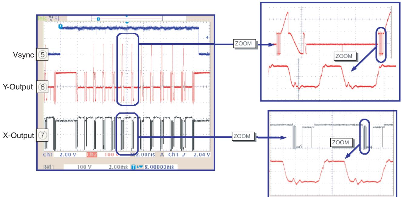
Figure 8-11 Waveform of X- and Y-board (42" SD v2)
