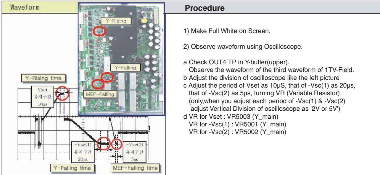
Figure 8-12 How to adjust the waveform (42" SD v2)
