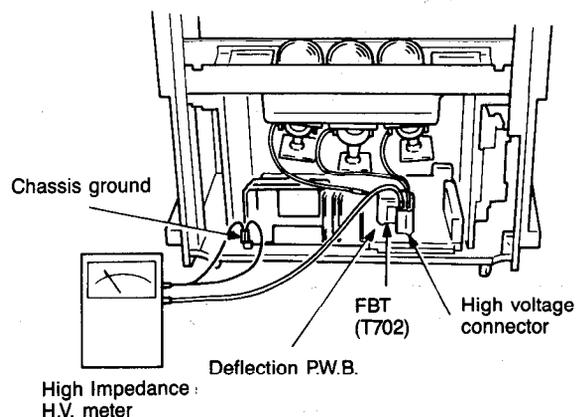
g. **X-radiation — TUBE:** The primary source of X-radiation in this receiver is the picture tube. The tube utilized for the above mentioned function in this chassis is specially constructed to limit X-radiation emissions.
