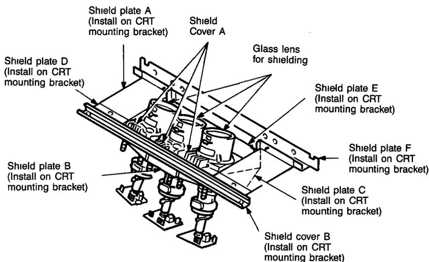
Detailing X-radiation shields
