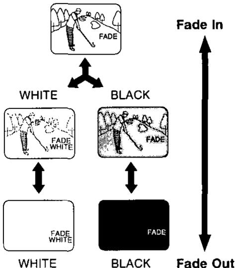
If FADE is accidentally pressed, simply press it again so that "FADE" disappears in the EVF.
