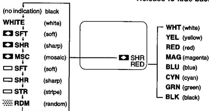
■ To create more effects: You can stop the fade at any time by pressing the **MODE SEL** button (other than BLACK, WHITE, and RANDOM modes). Pressing the **FADE** button will continue the fade.
