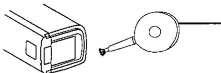
**3** Remove any lint or dust particles with a blower, available at photography stores. Do not touch lenses with fingers. Then, replace the eyepiece.
