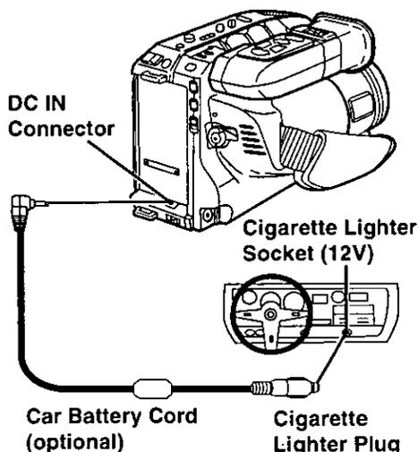
**1** Connect a PV-C16 Car Battery Cord (optional) to DC IN on the Camcorder.
