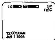
**2** Press DISPLAY once to change the display to date only. Press once or twice more to remove the date/time display.
