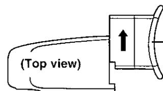
**2** Remove the eyepiece. (Do not twist.)
