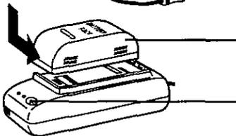
**2** Place the Battery into the AC Adaptor.
