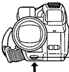
For Auto Focus mode, it may be necessary to press **MANUAL FOCUS**, so that "MF" does not appear in the EVF.
