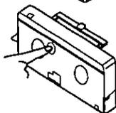
**2** Hold the PlayPak securely in one hand. Put your finger through the hole in the bottom of the PlayPak and push the cassette out.
