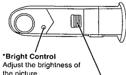
**\*Note:** These controls have been set at the factory. It is not necessary to adjust these controls under normal circumstances. But, should it become necessary, be careful to make the adjustment with a small, slender screwdriver so as not to damage the miniature control.
