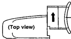
**2** Remove the eyepiece. (Do not twist.)
