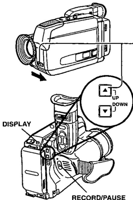
**1** While pressing the UP ▲ button, set the POWER switch to CAMERA.
