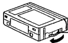
**1** Turn the **Tape Wheel** in the direction of the arrow until there is no slack.
