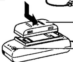
**2** Place the Battery into the AC Adaptor.
