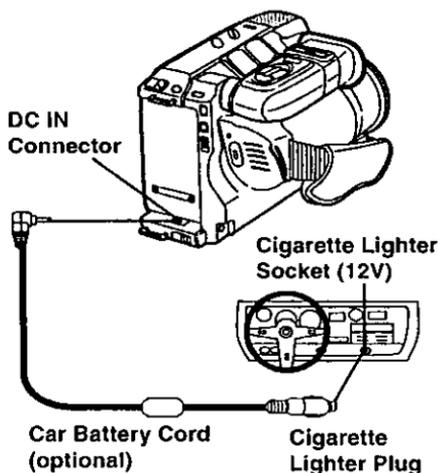
**1** Connect a PV-C16 Car Battery Cord (optional) to the DC IN of the Palmcorder.
