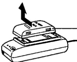
**3** Press the BATTERY REFRESH button. The CHARGE Lamp will flash when discharging begins and stop flashing when fully discharged. POWER Lamp will stay lit when fully charged.
