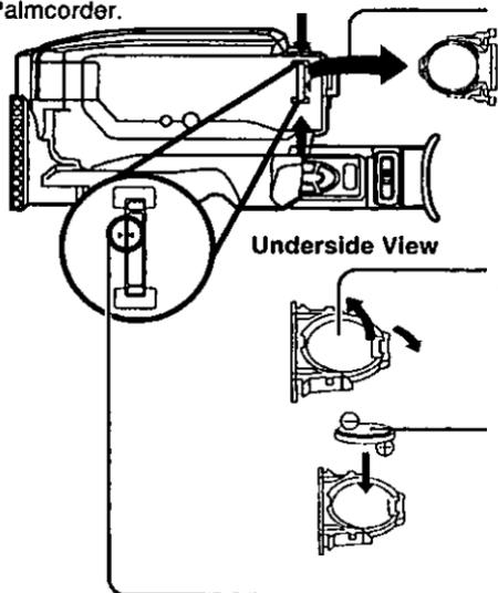
**1** While pinching the stopper tabs, pull the tray out of the Battery Compartment.
