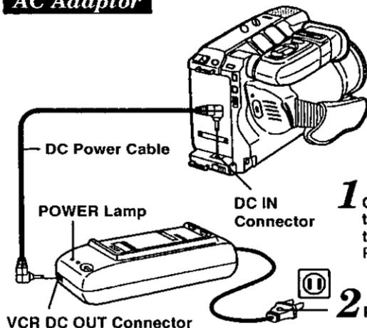
**1** Connect the VCR DC OUT on the AC Adaptor to the DC IN on the Palmcorder with the DC Power Cable (supplied).
