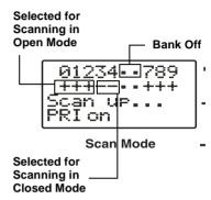
To turn on banks while scanning, press the number key until the bank's number appears. For example to turn bank 1 on again, press 1.
