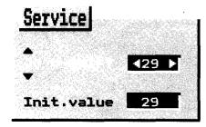
In service mode an adjustment menu is shown on the screen. The adjustment number and name, initializing (bottom) and adjustment (top) values are shown in the menu.
