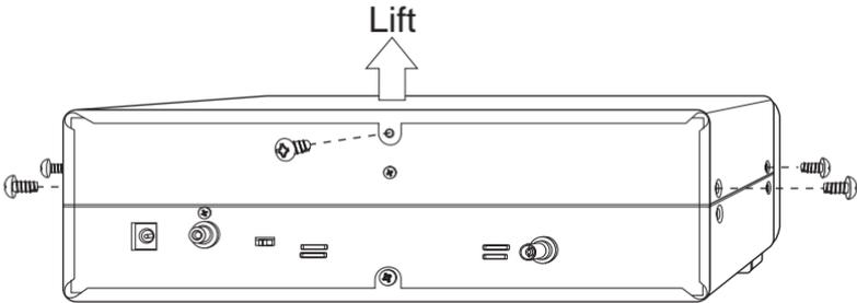
2. Carefully lift the cover up from the back of the unit and turn it to the left - being careful not break the speaker wire.
