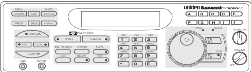
Programming, Search, Scan, Mode, and Numeric Keys, and Rotary Tuning Controls
