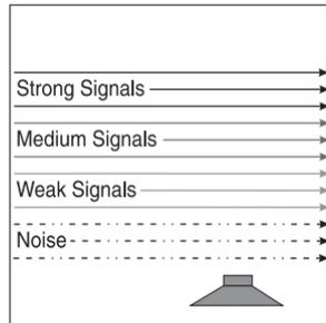
4. Turn **SQUELCH** back counter clockwise just until the hiss stops. Now the “Squelch Gate” allows only strong signals through.
