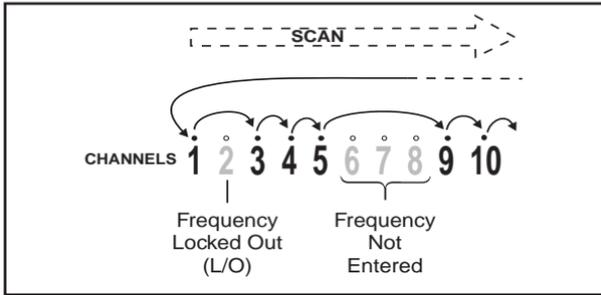
An optional DELAY can be set so that the scanner stays on the channel for 2 more seconds, waiting for another transmission before resuming scanning.
