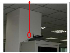
Please don't install the base unit next to the wall or pillar (concrete obstacles) → incorrect installation
