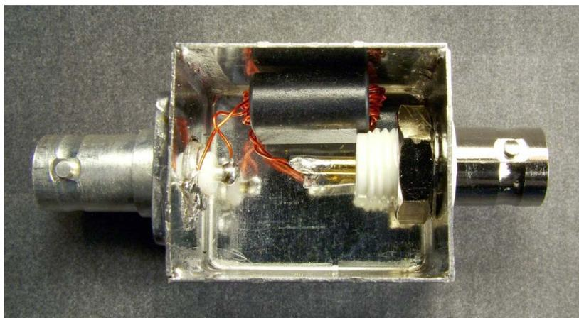
Figure 2.26 RF current choke housed in a small metal box. Note the isolated BNC connector on the right hand side
