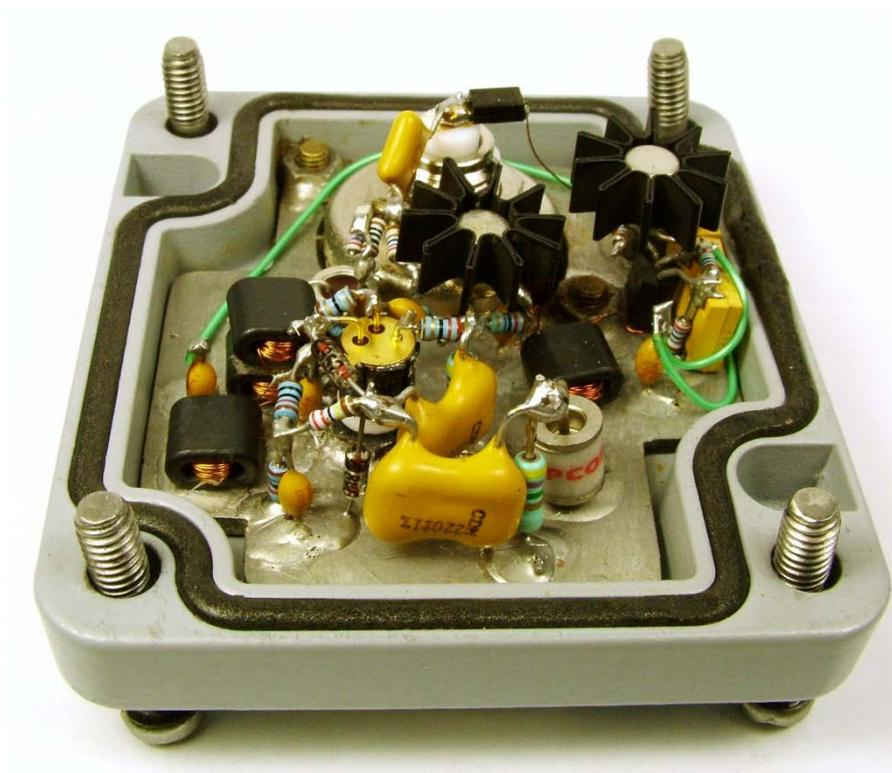
Figure 2.19 Point to point wiring of the active antenna. The two yellow series connected silver mica capacitors are in the foreground
