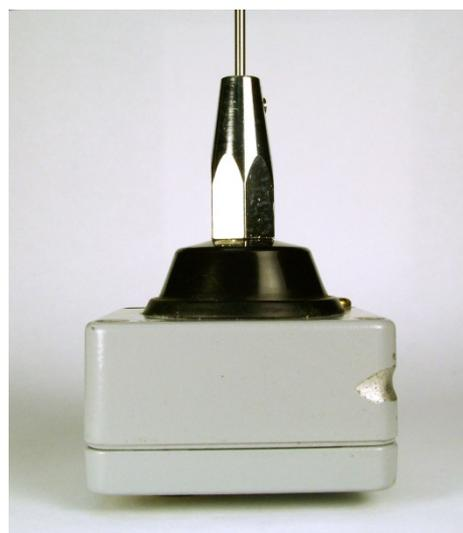
Figure 2.21 Assembled antenna with rod
