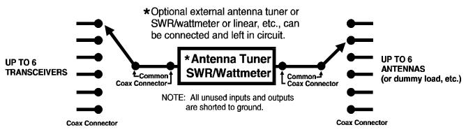
CONNECT ANY TRANSCEIVER TO ANY ANTENNA.
